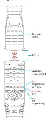
5. Press the desired button on your TV remote control for 2-3 seconds. Once the signal has been received, the red illumination of the TV-Control-Button will disappear and blink 3 times afterwards if the programming was successful or 10 times if
