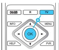
2. Enter 777 using the Numeric Keypad to start the search mode. During the process point the IR-Sensor in the direction of your TV.
