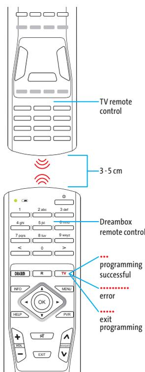
5. Press the desired button on your TV remote control for 2-3 seconds. Once the signal has been received, the red illumination of the TV-Control-Button will disappear and blink 3 times afterwards if the programming was successful or 10 times if
