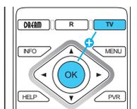
2. Press 888 on the Numeric Keypad to activate the learning mode. The blue illumination of the keys will turn off and the TV-Control-Button will light up red.
